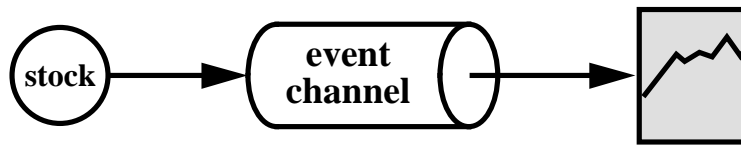
Figure 2 An event channel is an object service that decouples communication among distributed objects.
